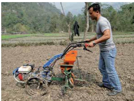
Designed and developed power tiller operated two row multi-crop seed drill cum planter
