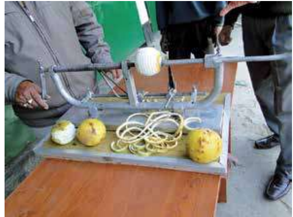
Mechanical Citrus macroptera peeling machine
