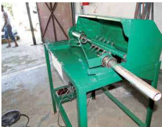
Mechanical Bamboo Shoot Peeling machine
