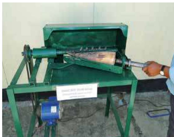
Mechanical Bamboo Shoot Peeling machine
